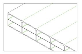
**TEKNOMULTI PC** is the multiwall polycarbonate sheet manufactured by SKRIMIZEAS SA The sheet is characterised hiah optical clarity, by light transmission, impact resistance and durability. It is available in a range of standard sizes, clear and tinted. TEKNO MULTI PC Longlife has a coextruded UV protection layer on one side.
